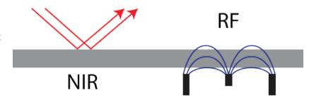
The PMT-330 is available in two options to accurately measure moisture of different board thicknesses:
